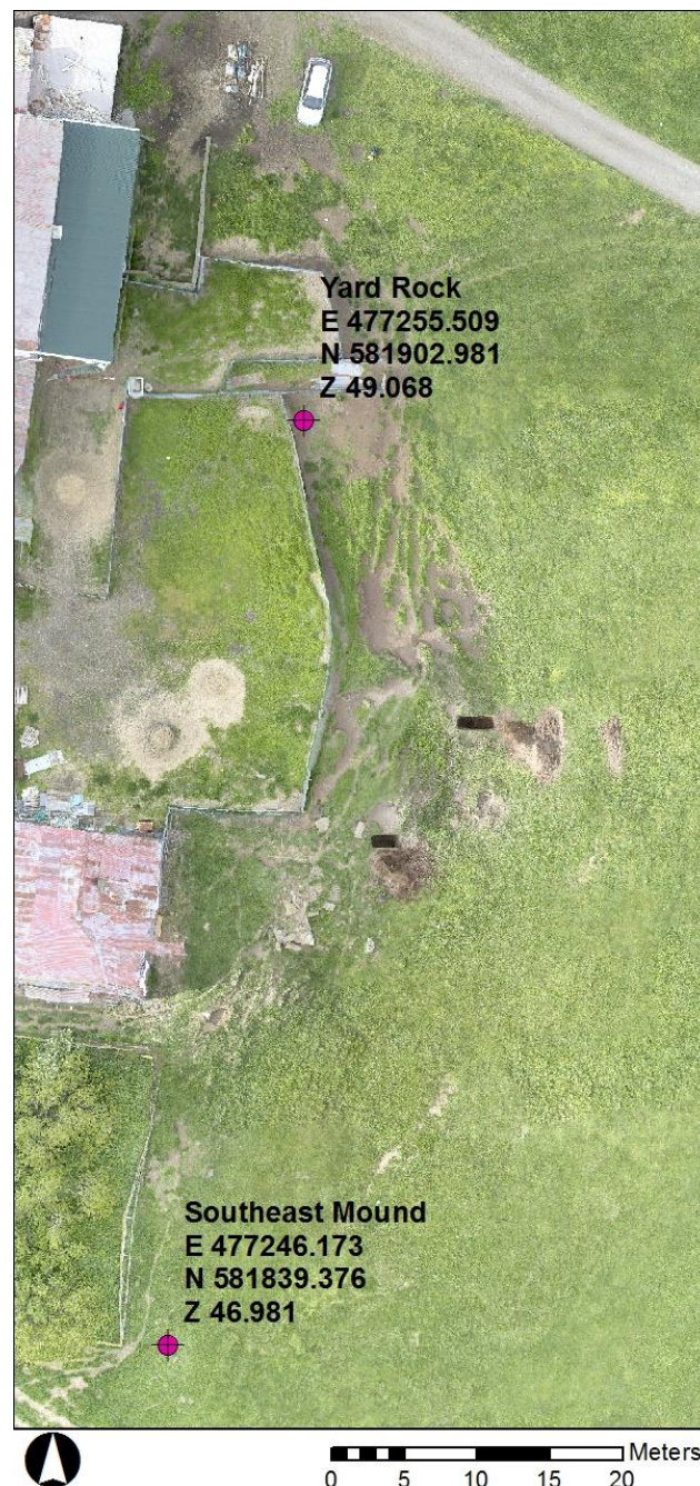
Figure 33. GNSS measured base points for total station set up.
