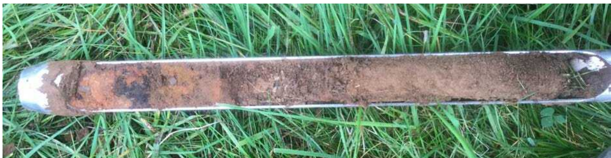
Figure 26. Core 163935 showing floor from 30-47 cm bgs (which continued into the next core barrel). Above the floor was an 8 cm LDC deposit with an in situ H1 at 21 cm bgs. The floor rested on gravel at 47 cm bgs.
