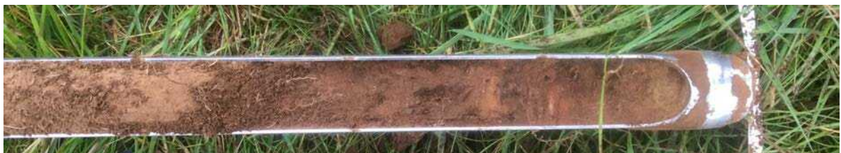
Figure 23. Core 163924 showing floor from 28-31 cm bgs. Below the floor was 24 cm of aeolian deposits, which had an in situ H3 at 39 cm bgs. The aeolian deposit bottomed out on gravel at 55 cm bgs.
