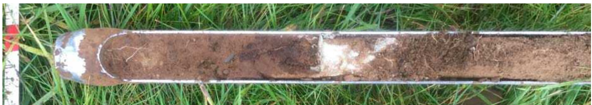
Figure 22. Core 163923 showing LDC from 27-45 cm bgs, clearly under an in situ H1 at 20 cm bgs. Below the LDC was 3 cm of aeolian deposit, which bottomed out on gravel at 48 cm bgs.
