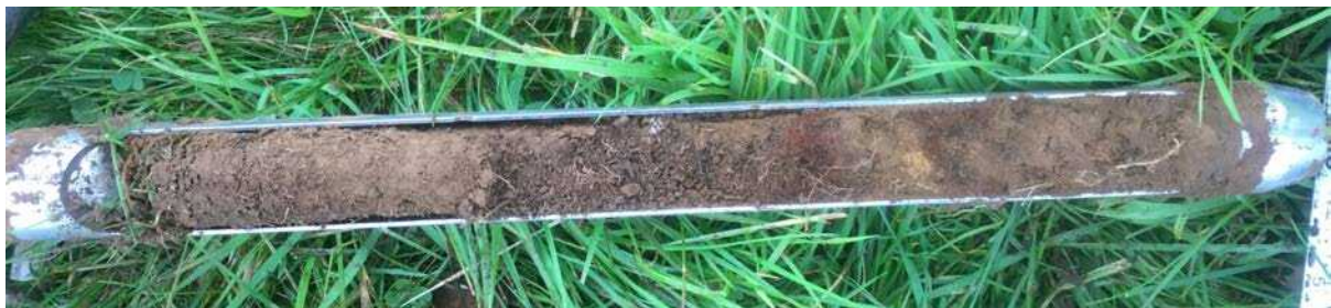
Figure 25. Core 163927 showing Turf from 20-37 cm bgs, under an ephemeral in situ H1 (visable in the center of the core at the top) at 16 cm bgs. Below the turf was 4 cm of aeolian deposit (which contained in situ H3/H4)), which bottomed out on gravel at 41 cm bgs.
