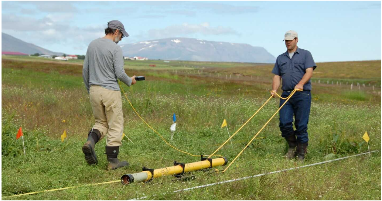
Figure 7. Electromagnetic surveying with the DualEM-21 (pictured at Stóra-Seyla). Damiata, keeps track of the distance, while Steinberg right, pulls unit at an even pace along the ground surface.
