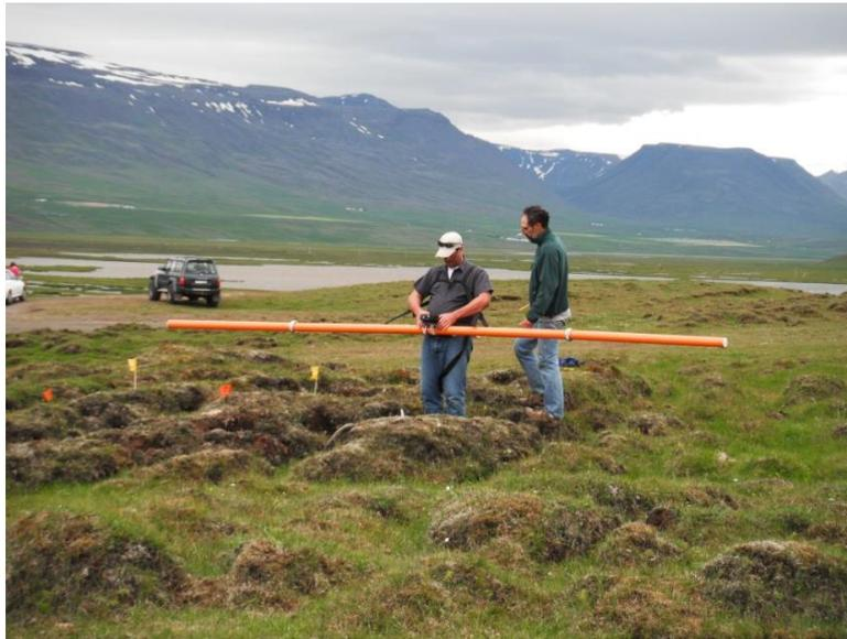
Figure 2. Using the CMD Explorer with the boom oriented perpendicularly to the direction of transects.
