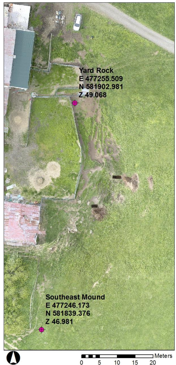
Figure 23. GNSS measured base points for total station set up.
