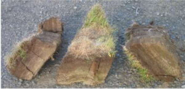
Wedge-shaped klömbruhnaus turf pieces.
